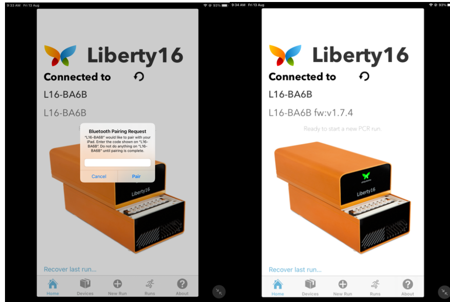
Figure 7: Liberty16 Home Screen with pairing request and after pairing is complete – Device name is shown. To change connected device, tap on My Devices at the bottom of the screen.
